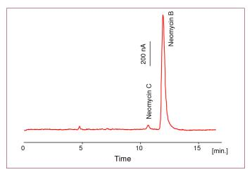
**Figure 3:** Example chromatogram of a 75 μg/mL Framycetin sulphate reference standard solution (EP BP190 –F67029), 10 μL injected (Note that chromatogram 1b was recorded with slightly different LC conditions as 1a).
