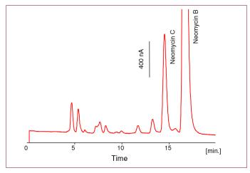
**Figure 2:** Chromatogram of a 0.5 mg/mL solution of commercial Neomycin sulphate formulation, 10  $\mu$ L injected. Neomycin B is the main constituent and neomycin C the main impurity.
