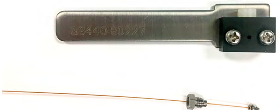
Figure 7. Thread the column through the internal nut, ferrule, and swaging tool
