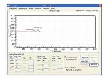
Analysis results showing stability on 19 consecutive cycles for  $H_2S$  & COS at concentration of 400ppb. Then switch on span gas at 10ppm for  $H_2S$  & COS, then switch on zero gas for  $H_2S$  & COS.
