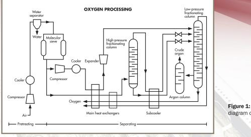
Figure 1: diagram of a cryogenic distillation process
