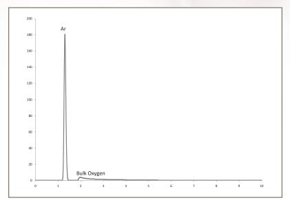
Figure 3: 1 ppm Argon in pure Oxygen
