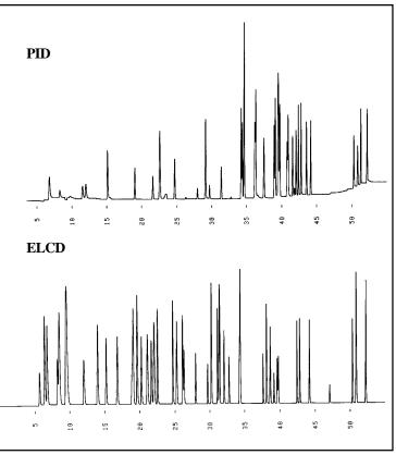
Figure 5. Rtx-502.2 Column, 105 m x 0.53 mm I.D. X 3.0 µm Film Using the Manufacturer's Recommended GC Program and an OI Analytical PID/ELCD Tandem Detector (5 mL of a 20-ppb 502.2 Standard). This Column Requires the Longest GC Run Time for Complete Peak Separation, but it Makes Use of OI Analytical's Economical and Unique Tandem PID/ELCD.
