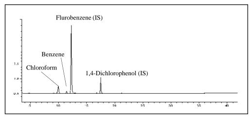
Figure 14. Chromatogram of River Source Water for a Water Utility Run on the AMPS and the Model 4560. This Fully Automated System was Configured to Monitor for 21 Key Compounds at Single-Digit ppb Levels as well as for Increases in Total VOC Concentrations.
