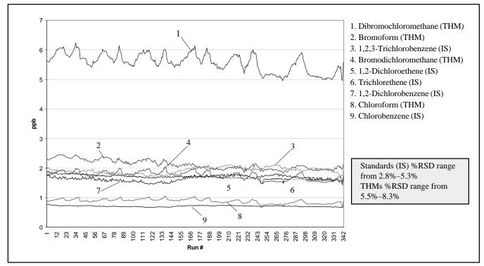
Figure 15. Results for Both the THMs and the Internal Standards (IS) when using the Optional Standards Addition Module (SAM). The SAM was Programmed to Add the IS During each Analysis. The Stability of the Standard Response over Seven Days Verifies that the Changes Observed in the THM Concentration are Actual Minor Changes in their Concentration in the Tap Water and not Caused by any Purge and Trap/GC Related Drift.
