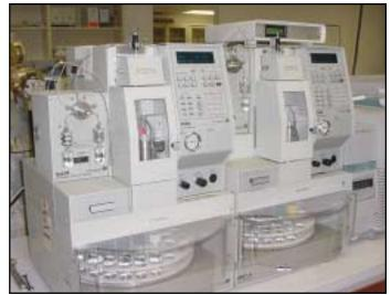
Figure 9. OI Analytical Dual Purge-and-Trap System Using the PT Express and SAM
