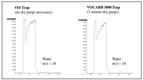
Figure 2. Water Profile on an OI Analytical #10 Trap and on a VOCARB 3000 Trap. The Model 4560 Patented Cyclone Water Management System Effectively Removes Most of the Water Retained on the #10 Trap, Making the Volume of Water to the GC Column Comparable to that Retained on the Hydrophobic VOCARB 3000 Trap, about 0.25 µL.
