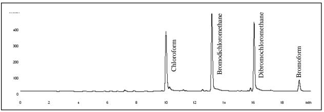
Figure 13. A Representative Chromatogram of THMs Collected During Continuous Monitoring of Local Tap Water Using the AMPS. The Analysis was Performed on an OI Analytical Halogen Specific Detector (XSD<sup>™</sup>), which Responds Only to the Halogenated Compounds Present in the Sample. The Only Peaks that are Observed in this Analysis are Low ppb Levels of the THMs.
