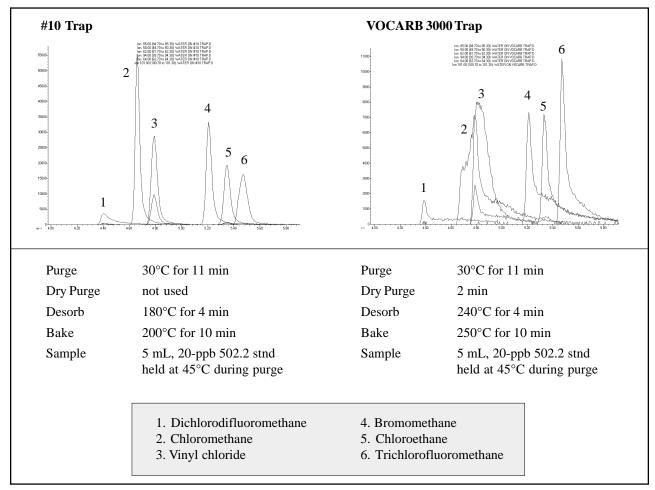
Figure 1. First Six Gases on an OI Analytical #10 Trap and on a VOCARB 3000 Trap. The Steam-Driven Pressure Pulse of the #10 Trap Improves Chromatographic Peak Shape for These Six Early Eluting Compounds When Run on the Model 4560. Both Traps were Preconditioned and Operated According to the Manufacturer's Instructions.
