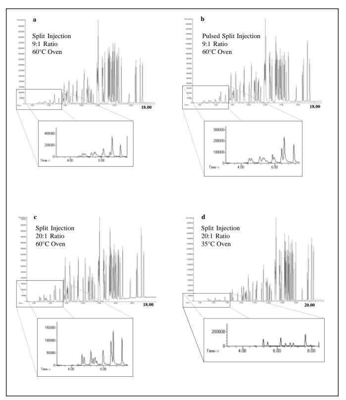
Figure 7. Rtx-VMS Column, 60 m x 0.25 mm I.D. x 1.4 µm film, Shown Using Several Different GC Programs (5 mL of a 20-ppb 502.2 Standard). This Column is Nearly Identical to the Column Used for Figure 6, and the Reduced Analysis Time is due to a Faster GC Oven Program. This Column is now a Best Seller and has Reduced GC Analysis Time to Between 18 and 21 Minutes.
