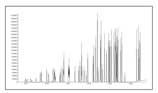
Figure 6. DB-VRX Column, 60 m x 0.25 mm I.D. x 1.4 µm film, Using the Manufacturer's Recommended GC Program (5 mL of a 20-ppb 502.2 Standard). This Column has set the Benchmark for Many Years with an Analysis Time of About 33 Minutes and Made the GC Run the Rate-Limiting Step in VOC Analyses.
