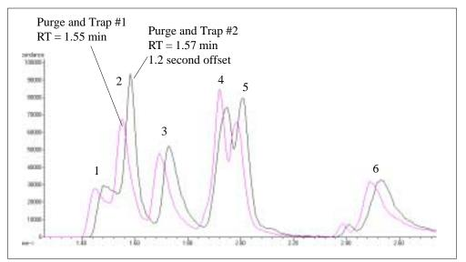
Figure 10. Early Eluting Peaks, Such as These Six Gases, will have a Slight Retention Time (RT) Offset of About 1 to 1.5 Seconds due to the Longer Transfer Line for the Second Purge and Trap. This RT Offset can be Used as a QC Tool to Help Identify Which Purge and Trap a Given Sample was Run on. The RT Offset is Not Observed for the Later Eluting Compounds.
