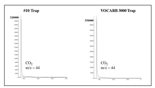
Figure 3.  $CO_2$  Profile on an OI Analytical #10 Trap and on a VOCARB 3000 Trap. Significantly less  $CO_2$  is Generated by the #10 Trap and Transferred to the GC than with the Carbon-Based Adsorbents in the VOCARB 3000. This Reduction in  $CO_2$  Further Improves Chromatographic Performance of the Early Eluting Compounds.
