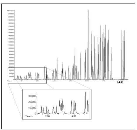
Figure 8. DB-VRX Column, 20 m x 0.18 mm I.D. x 1  $\mu$ m film, Using the Manufacturer's Recommended GC Program (5 mL of a 20-ppb 524.2 standard). This Column has Reduced the GC Analysis Time to as Little as 15 Minutes, Making the Purge-and-Trap Cycle Time the Rate-Limiting Step.
