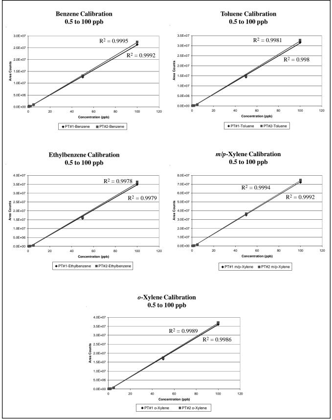
Figure 11. Calibration Curves for all Five BTEX Peaks on Two Matched Purge-and-Trap Units of a PT Express. Note the Excellent Agreement Between the Two Curves for Each Compound and the Nearly Identical Correlation Coefficients, Demonstrating How Well the Two Units are Matched.
