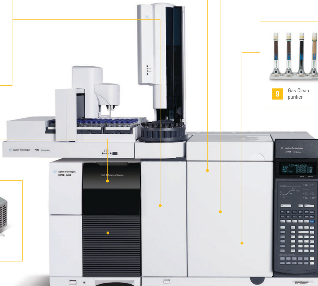
2 Inert Flow Path Split/Splitless inlet
