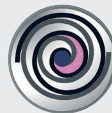
Gas exhausted at center hub
