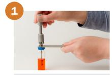
**Probe insertion:** Two probe lengths allow immersive or headspace sampling in 20 or 10 mL vials.
