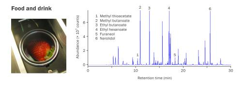
**Aroma-profiling foods and beverages** is widely studied using TD. In this example, Markes' Micro-Chamber/Thermal Extractor is used to quickly profile a range of aroma compounds from strawberries in a single run.
