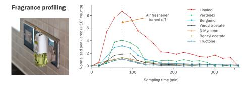
**Analysis of fragranced products** is another important application of TD, and Markes' on-line systems offer the additional advantage of continuous monitoring. This is used here to track changes in airborne components from a plug-in air-freshener.
