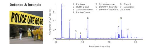
**In homeland security and forensic applications**, TD is used to detect a wide range of analytically challenging chemicals – including chemical agents, explosives, drugs of abuse, fire accelerants, and products of body decomposition (shown above).
