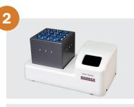
**Analyte extraction:** The HiSorb Agitator efficiently mixes and heats the sample.
