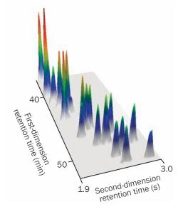
The high spectral acquisition rate of BenchTOF results in excellent peak shape and peak-to-peak resolution for challenging GC×GC analyses, such as this set of dichloroto heptachlorobiphenyls.
