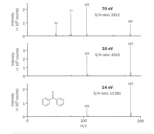
**The ability of Select-eV to enhance the molecular ion** stands out in this set of spectra for benzophenone (MW 182). Note the enhancement of sensitivity at lower ionisation energies, and the ability to optimise intensities of fragment or molecular ions by a slight change in the energy used for soft ionisation.
