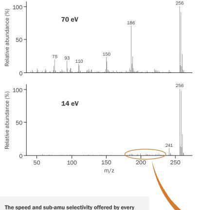
BenchTOF is complemented by the ability of Select-eV to detect and visualise co-eluting components. In this GC×GC analysis of PCB-29, the complexity of the 70 eV spectrum makes it difficult to visualise minor impurities. The reduced fragmentation at 14 eV makes it easy to detect and deconvolve these components.
