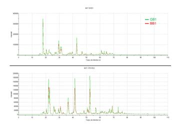
Fig 2. Heracles e-nose chromatograms of yerba mate optimal and less optimal quality samples
