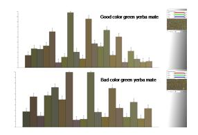
Figure 7.Color spectrum comparison for the good and bad green yerba mate batches
