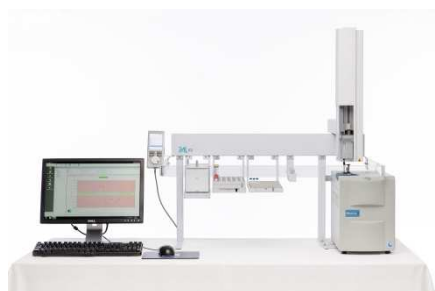
Fig. 1: Ultra Fast GC based HERACLES Electronic Nose
