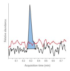
The SRM ion chromatogram of verapamil (MRM transition  $455.3 \rightarrow 164.9$ ) for 100 attograms (200 zeptomoles) injected on-column (blue). The red trace shows a blank injection.
