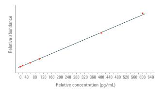
Linear response of verapamil from 100 attograms to 100 picograms injected on-column. The  $\rm R^2$  value (0.997)underscores the wide range of linear response.
