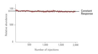
Data shows consistent peak response for 2,000 consecutive injections of verapamil in plasma (20 femtograms injected on-column)—more than four days of continuous operation. RSD for the peak area is <6%. Normally, peak-area stability in plasma is shown for picogram quantities injected on-column; levels in this example are more than one hundred times lower.
