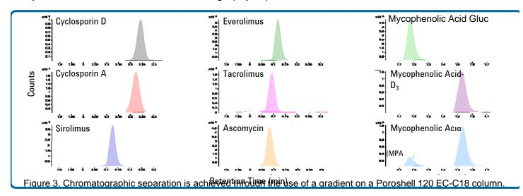
Due to the presence of mycophenolic acid glucuronide (MPA-G) in plasma, chromatography is particularly important to the analysis of mycophenolic acid. MPA-G is susceptible to in-source fragmentation where glucuronide is easily lost. If these analytes are not separated by retention time, deglucuronidated MPA-G (MPA-G\*) can falsely elevate the determination of mycophenolic acid concentrations.
