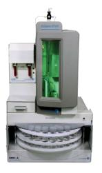
The **4551A Autosampler** docks directly underneath the Eclipse 4760 and enables unattended automated analysis of 51 water samples. The 4551A can be equipped with options for cooling sample vials and adding internal standards to ensure compliance with quality control requirements in USEPA methods. The optional **LV-20 Standards Addition Module** is equipped with high-speed injection valves that minimize standard usage and help decrease laboratory operating costs for expensive standards.
