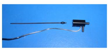
Figure 32 Ferrule Placement on Lower Burner Tube
