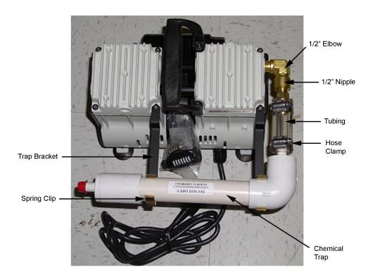
Figure 15 The Welch Dry Piston Pump
