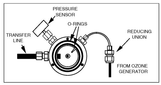
Figure 24 Reaction Cell
