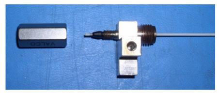
Figure 29 Positioning the Upper Tube in the Union Fitting
