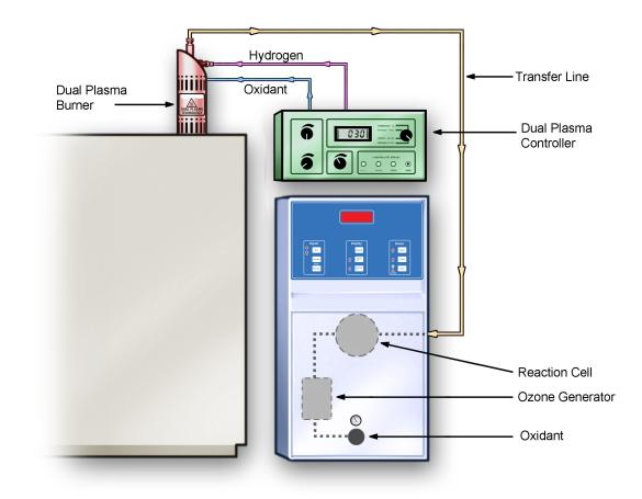
Figure 10 Drawing of the Detector with Dual Plasma Burner and Controller
