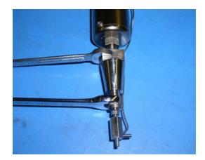
**Figure 41** Tightening the Heater Swivel Nut
