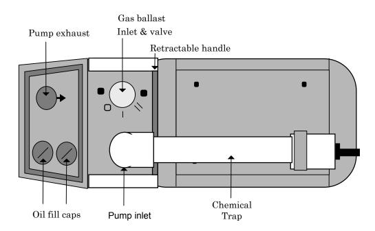
Figure 13 RV5 Oil- Sealed Vacuum Pump and Associated Traps (Top)
