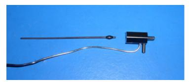
Figure 25 Ferrule Placement on Lower Burner Tube
