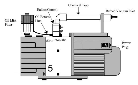
Figure 12 RV5 Oil-Sealed Vacuum Pump and Associated Traps (Back Side)
