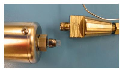
Figure 44 Large Quartz Tube Properly Inserted into the Quartz Heater Assembly
