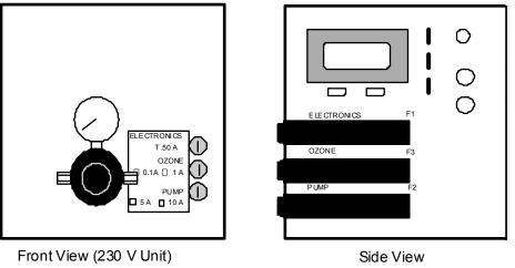
Figure 47 Fuse Positions on the Power Supply Board
