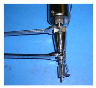
**Figure 30** Tightening the Heater Swivel Nut
