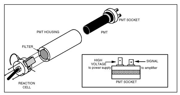
Figure 23 Reaction Cell, PMT Housing and PMT Socket
