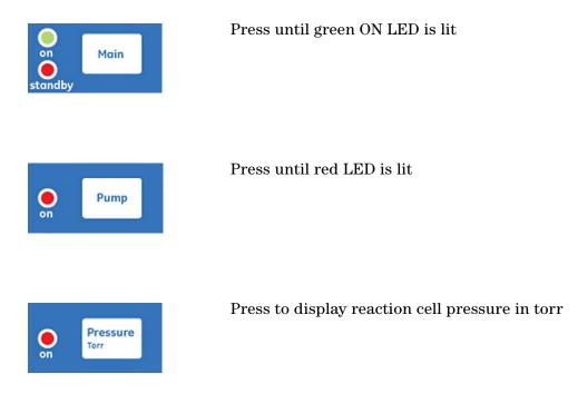
After the pressure has stabilized ( $\sim 5$  minutes), record the pressure below. Typical pressure in the reaction cell should be 1-2 torr with the oil-sealed pump, or 5-8 torr for the oil-free pump.
