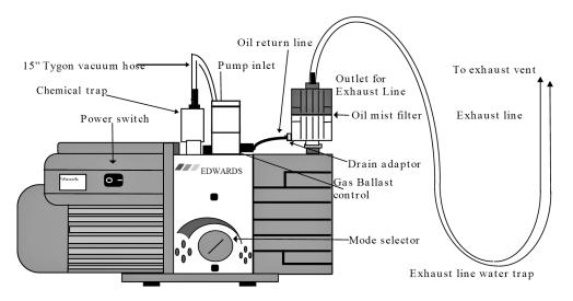
Figure 14 RV-5 Oil-S ealed Vacuum Pump Exhaust Line
