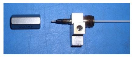
Figure 38 Positioning the Upper Tube in the Union Fitting
