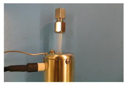
Figure 46 NCD Tube Replacement Detail
