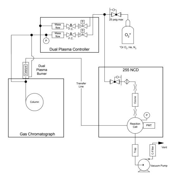
Figure 9 Schematic for 255 NCD, in Nitrosamine Mode
