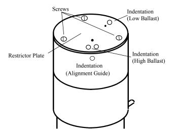
Figure 16 Oil Drain Kit with Ballast Control
