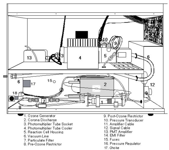
Figure 5 255 NCD Left Side View
