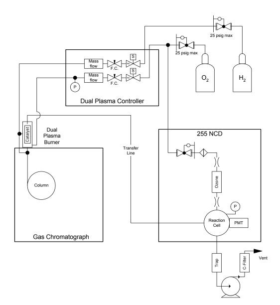
Figure 8 Schematic for 255 NCD, in Nitrogen Mode
