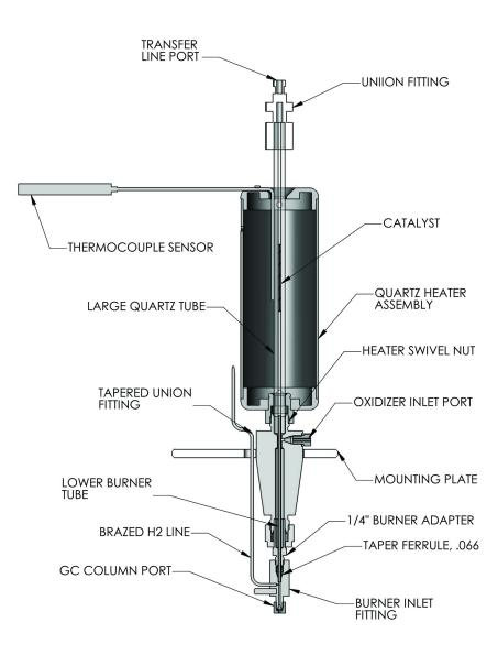
Figure 2 Cross-Section of the Dual Plasma Burner for the 255 NCD
