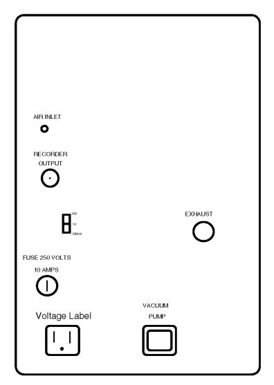
Figure 17 SCD (230 V Unit) Rear Panel Diagram
