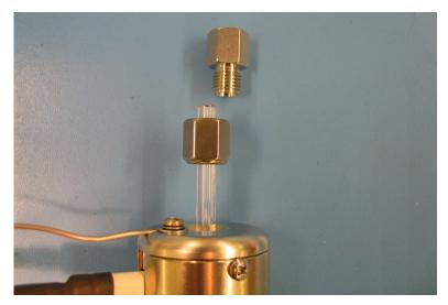
Figure 45 NCD Tube Replacement Detail
