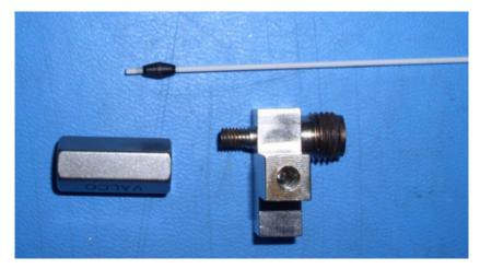
Figure 37 Orientation of the Double Taper Ferrule
