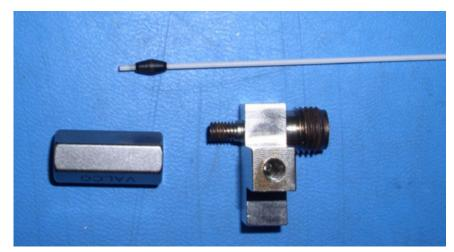
Figure 28 Orientation of the Double Taper Ferrule
