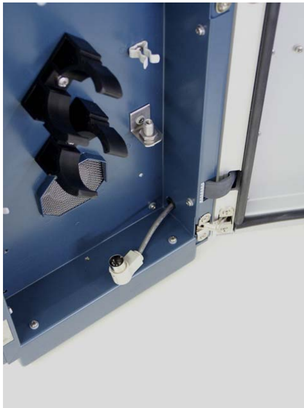
Figure 6. Installation of valve-to-module cable inside DECADE II.
