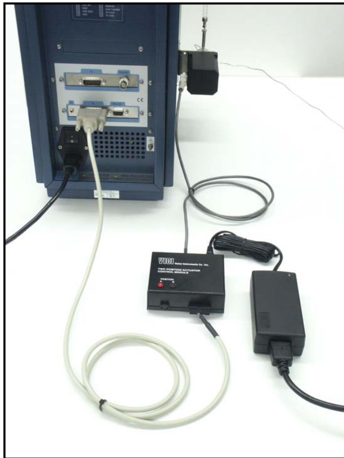
Figure 14. Cable connections DECADE II to valve.
