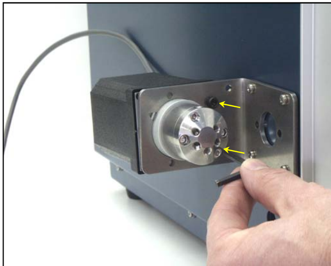
Figure 13. Securing valve in external valve bracket.
