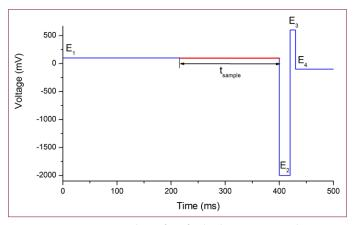
$\textbf{Figure 3:} \ 4\text{-step PAD potential waveform for the detection FDG and impurities}.$
