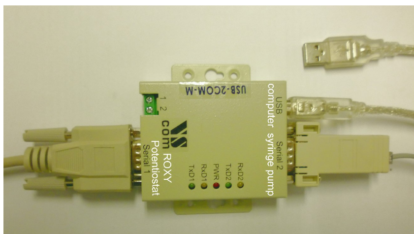
Fig. 5. Photo of the USB – RS232 converter with serial cables from potentiostat and syringe pump connected to Serial 1 and Serial 2, respectively. Converter is connected to computer using an USB port.
