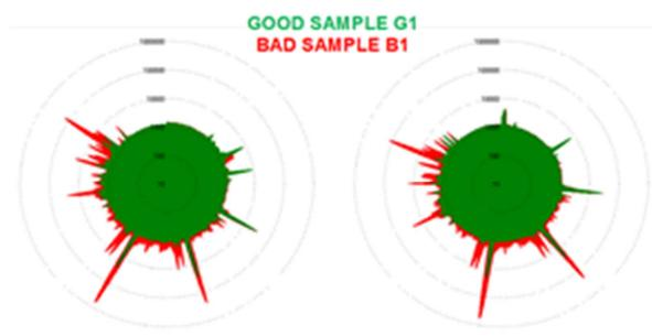
Fig. 1: Radar plots (odor fingerprints) of G1 (good) and B1 (bad) samples of polyethylene obtained with the chromatograms of HERACLES II on the 2 columns
