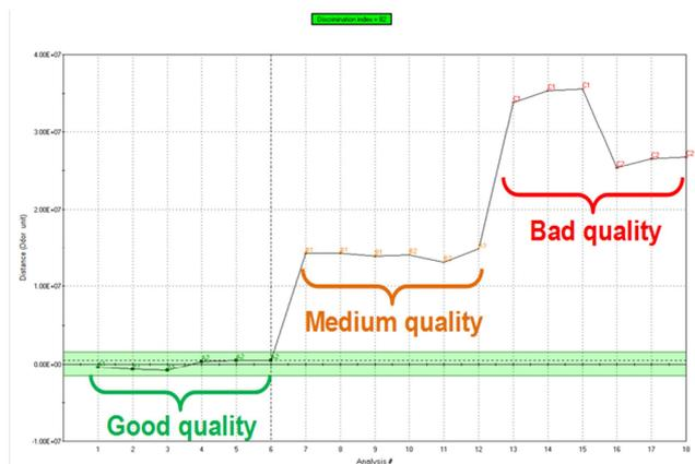
Fig. 4: Statistical Quality Control model of polyethylene pellets obtained with the major peaks measured with HERACLES e-nose
