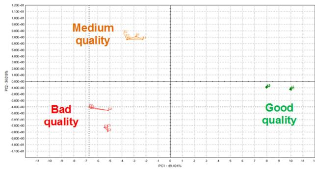
Fig. 3: Principal Components Analysis of polyethylene pellets obtained with HERACLES e-nose measurements
