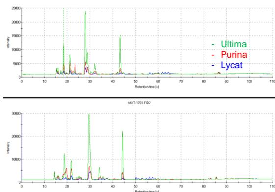
Figure 4: Superimposed chromatograms of the 3 brands of Pet food, obtained with HERACLES NEO e-nose
