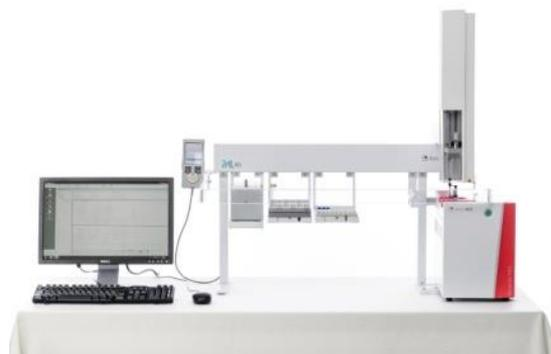
Figure 1: Ultra-Fast GC based HERACLES NEO Electronic Nose (Alpha MOS, France)
