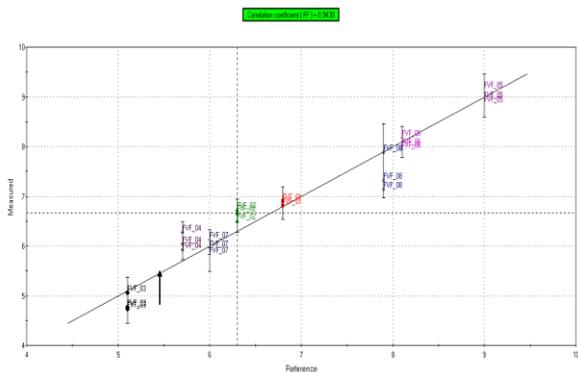
Fig. 6: Correlation model between sensory panel and e-nose measurements based on PLS (Partial Least Square) model
