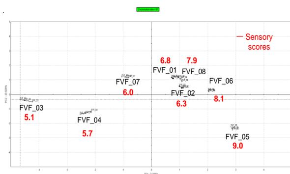
Fig. 5: Principal Components Analysis of sunflower oils obtained with HERACLES e-nose measurements
