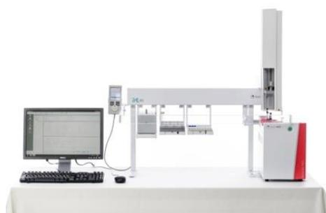
Fig. 1: Ultra Fast GC based HERACLES Electronic Nose (Alpha MOS, France)
