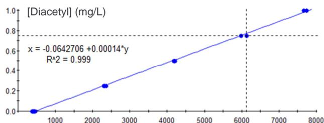
Figure 3. Calibration curves of diacetyl in orange juice on Heracles II e-nose on MXT-5 column
