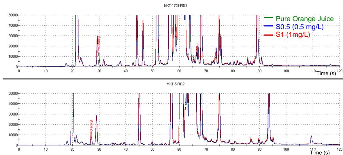
Figure 2. Chromatograms of orange juice with and without addition of diacetyl obtained on the 2 columns of HERACLES e-nose
