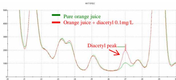
Figure 4: Comparison of the chromatograms of pure orange juice and orange juice with addition of 0.1 mg/L (100 ppb m/v) of diacetyl obtained on column MXT-5 of HERACLES
