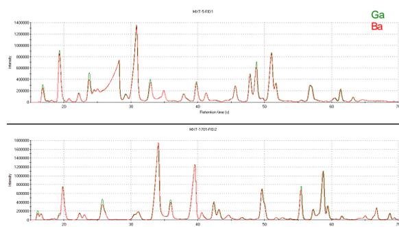
Fig. 3: Zoom on chromatograms of 1 good quality coffee batch and 1 coffee batch stored in stressed conditions
