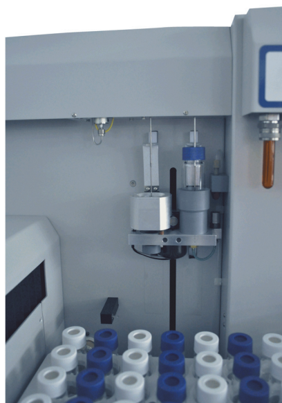
Figure 6. 4100 Sampling Station with Lift Mechanism Raised
