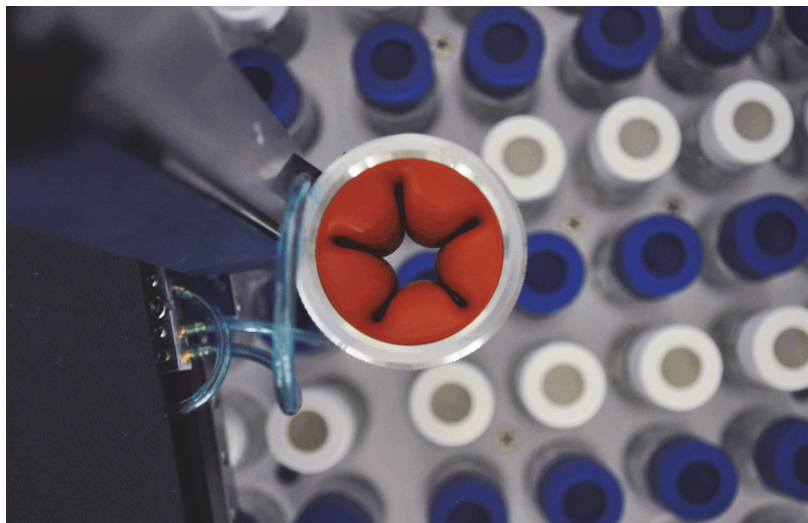
Figure 3. VOA Constrictor™ Vial Gripper Mechanism Pressurized without Vial
