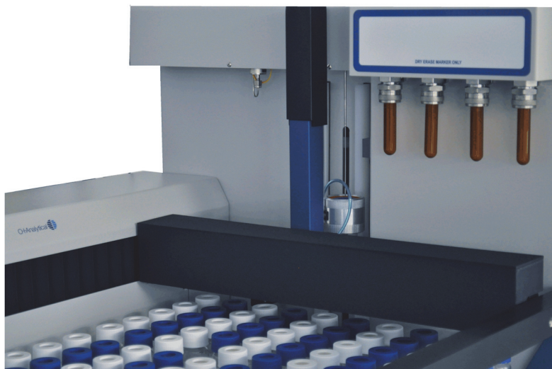
Figure 5. Standards Addition Manifold with Dry Erase Panel
