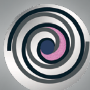
Gas exhausted at center hub
