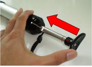
d) When the flow has stopped, rotate the plunger dot away from the pump-shaft alignment mark a ¼ turn either to the right for 100 mL sample volume or to the left for 50 mL sample volume.
