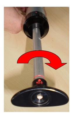
e) For additional pump strokes, push the handle back fully without removing the tube from the pump then repeat steps c and d. The number of strokes taken can be recorded by rotating the counter on the pump.
