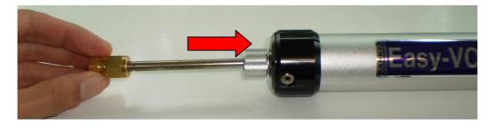
b) Align the red dot on the pump shaft with the 50 mL or 100 mL sample volume red dot on the plunger. Pull the plunger one full stroke and wait 2 minutes. The plunger should still be held during this period.
