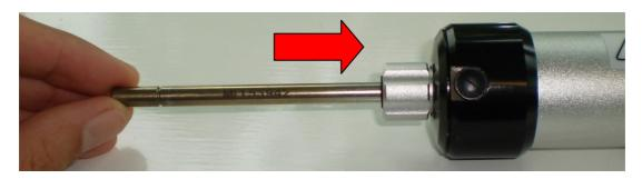
b) Select the sample volume required by aligning the red dot on the plunger with the pump shaft alignment mark.
