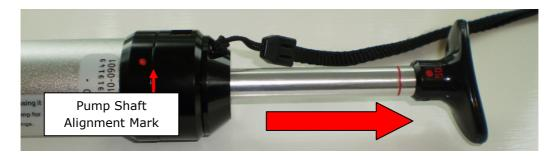
c) Rotate the plunger dot away from the pump-shaft alignment mark a ¼ turn to the right for 100 mL sample volume or to the left for 50 mL sample volume.
