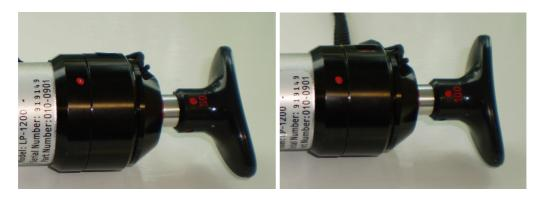
c) Pull the handle quickly until it latches at  $\frac{1}{2}$  or full stroke (50 or 100 mL) and wait, until the flow through the tube has stopped (typically 30 seconds).
