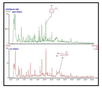
**Figure 1.** Switchgrass at 600°C, High pressure (top) and low pressure (bottom).
