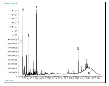
**Figure 1.** Pyrolysis of tire rubber at 700°C. Peak 1=butadiene, 2=isoprene, 3=butadiene dimer, 4=isoprene dimer, 5= 6-PPD, 6=Hydrocarbon oil.
