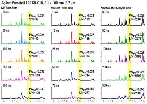
Agilent 1290 Infinity LC / 6410A Triple Quadrupole MS; Acetic Acid pH 3.8 / Acetonitrile Gradient, 1 mL/min; ESI+, Scan/SIM/dMRM, 350 °C, 10 L/min, 50 psi, 3500 V; Agilent Publication 5990-7824FN
