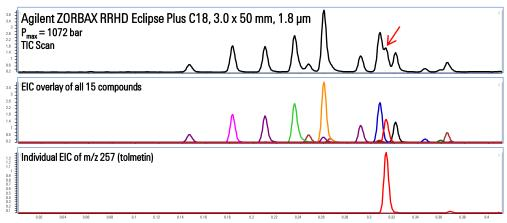
Agilent 1290 Infinity LC / 6410A Triple Quadrupole MS; Formic Acid pH 2.8 / Acetonitrile Gradient, 2.75 mL/min; ESI+, Scan 100-400, 350 °C, 12 L/min, 50 psi, 3500 V;
