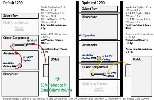
apillary, 0.075 x 340 mm capillary, 1.0 uL heat exchanger, 0.075 mm id needle seat: Ultra-Low Dispersion Max-Light Cartridge Flow Cell (G4212-60038)for UV analysi System Rack, 5001-3726; Agilent Publication 5990-9502EN
