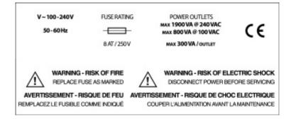
Replace blown fuses with fuses of proper type and rating as stipulated on the side panel and specified in the installation section of this manual. The fuse holder is integrated in the mains connector. Ensure that the instrument is never put in operation with fuses of a different type. This can cause fire.
