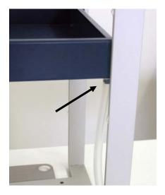
Leakage of solvent on the connectors on the back of the electrical equipment can lead to short circuit.
