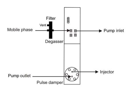
Fig. 6. LC connections OR 100/110.
