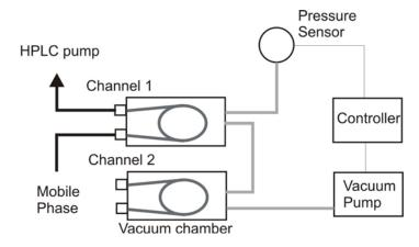
Fig. 12. Block diagram of OR 100 degasser
