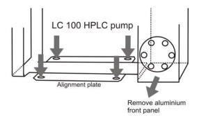
Fig. 4. Stacking LC 100 pump on OR 100 organiser rack.
