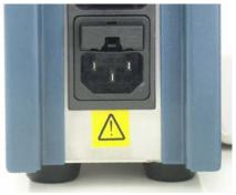
Connect the detector to a grounded AC power source, line voltage 100 – 240 VAC, frequency 50/60 Hz. The instrument should be connected to a protective earth via a ground socket. The power source should exhibit minimal power transients and fluctuations. Replace faulty or frayed power cords.
