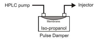
Fig. 13. Schematic representation of OR 100 pulse damper
