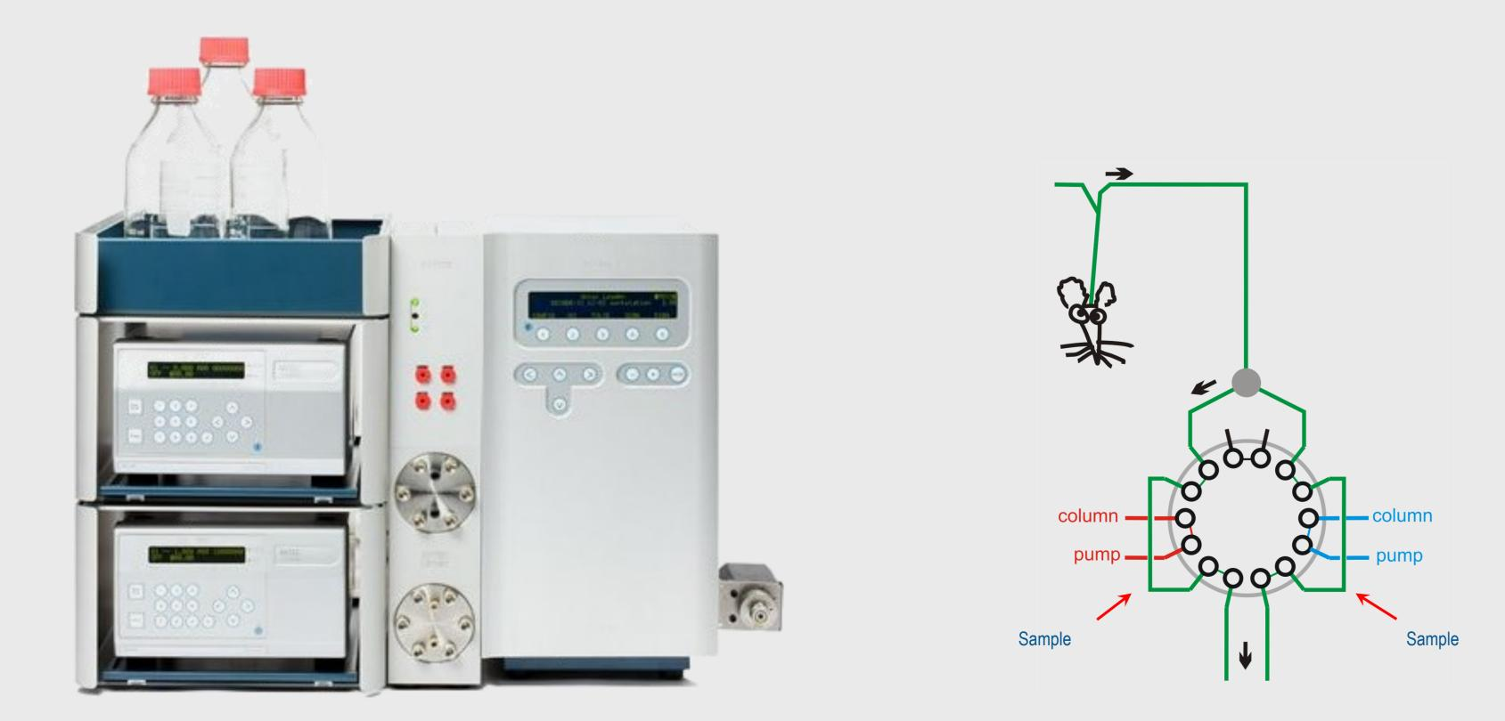
Figure 1. Left side: ALEXYS<sup>®</sup> OMD Analyzer for on-line in vivo microdialysis. Right side: Dual loop sampling valve for parallel analysis of Monoamines and Metabolites. During HPLC analysis the subsequent sample is loaded in the loop (no loss of sample/data).
