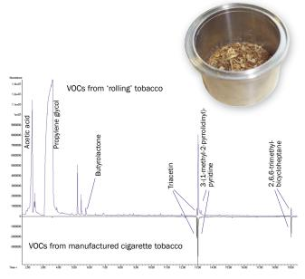
Vapour profiles from 'rolling' tobacco (top) and manufactured cigarette tobacco (bottom), collected on Tenax tubes using a μ-CTE at 50°C
