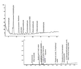
Emissions from wood veneer. Formaldehyde (HPLC) chromatogram (top) & VOC (TD-GC/MS) chromatogram (bottom)
