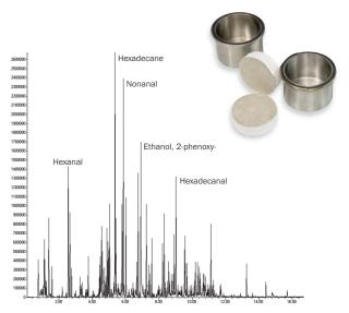
Screening of emissions from plasterboard (drywall)
