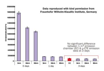
Area-specific emission rates determined for the  $\mu$ -CTE (blue) and an emission chamber (red) up to 3 days for a building product. Agreement is observed between the 2 methods at 3 days
