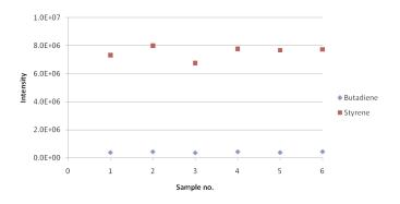
Precision of  $\mu\text{-CTE}$  chambers for ABS terpolymer samples showing responses for 1,3-butadiene and styrene
