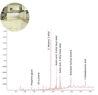
Surface emissions from a sample of vinyl flooring and adhesive tested using the  $\mu$ -CTE at 40°C with 50 mL/min air flow for 20 mins
