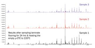
Step 2: ISO 16000-25 test carried out on 3 replicate samples of the same laminate flooring (area 4 x 3 x 0.8 cm)
