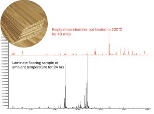
Step 1: Sample of laminate flooring analysed in 2 steps according to ISO 16000-25
