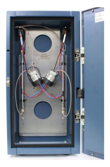
Fig. 13. DECADE Elite with 2 columns and 2 SenCell flow cells for parallel detection.
