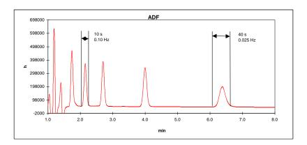
Fig. 21. Typical chromatogram with peak widths between 10 – 100 s.
