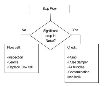
In case no significant drop in noise or cell current is observed service or replace the cell. In case you still cannot solve the problem contact your local representative.
