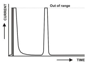
Fig. 48. Example of a chromatogram were the cell current exceeds the maximum current level and the signal is 'out of range'.
