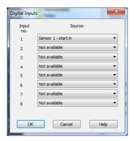
Connect the relay (contact closure) of the external device which functions as inject trigger to the 'digital IO connector on the rear panel of the detector to pin 21 (start 1) and pin 25 (ground). For sensor board 2 or 3 use pin 22 (start 2) and pin 23 (start 3) respectively.
