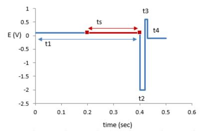
Fig. 29. Potential steps in pulsed amperometric detection. During t1 the detection potential is applied, detection occurs during ts. Steps t2, t3 and t4 are for regenerating the electrode. This process repeats itself continuously as soon as the cell is on.
