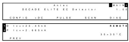
Fig. 14. DECADE Elite main menu (top) with active cell indicator in top right corner. Multi-STAT screen showing cell 1 (DC mode) and cell 2 (PULSE mode).
