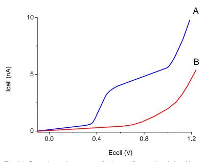
Fig. 34. Scanning voltammetry of 1.0 μmol/l norepinephrine (A) at a glassy carbon working electrode, at a scan speed of 10 mV/s. Scan (B) is the blank solvent.
