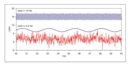
Fig. 22. Typical random noise in chromatography (lower trace). Both frequencies (0.4 and 10 Hz) can be recognised amongst others.
