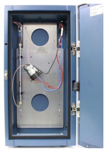
Fig. 4. Installation of flow cell and column in the DECADE Elite.
