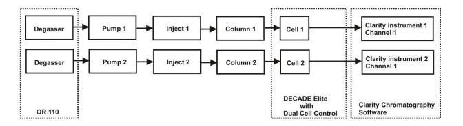
Fig. 12. Typical configuration for parallel mode detection. Two independent HPLC systems with dual channel support from OR 110, DECADE Elite and Clarity software.
