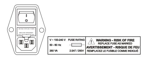
In case the fuses blow out repetitively contact Antec or its representatives for instructions and/or service of the instrument.
