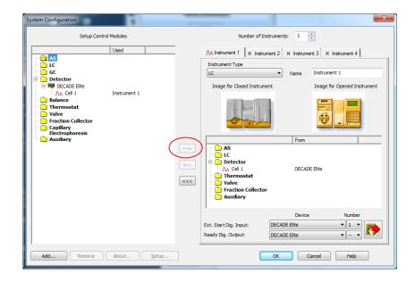
Add the DECADE Elite device to the Clarity instrument by clicking the right arrow button (encircled) and select Ext. Start. Dig. Input 'Device DECADE Elite, Number 1' to enable an external start trigger.
