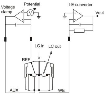
Fig. 9. Schematic representation of an electrochemical cell with a threeelectrode configuration.
