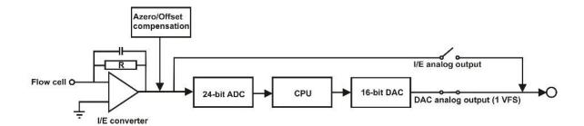
Fig. 46. Top: CONFIG screen. Bottom: DECADE Elite signal processing from electrochemical flow cell to output. R is a selectable I/E resistor of 100M, 10M, 10M, 10K or 1K in the I/E converter circuit.
