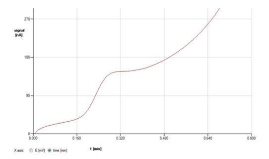
Fig. 42. Scan (cycle: half) of a 20  $\mu$ M Serotonin in mobile phase at a glassy carbon working electrode. Scan speed 20 mV/s.
