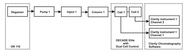
Fig. 11. Typical configuration for serial mode detection. Cell 1 is a FlexCell, cell 2 is a SenCell for detection. Channel 1 and 2 use the same time base of system 1.
