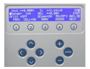
Fig. 6. DECADE Elite keyboard. The cursor is on 'Range' which allows changes using the value buttons '+' and '-'. The 'Enter' button is only used to confirm changes in potential (Ec) and range.
