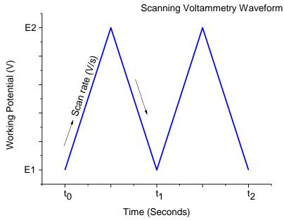
Fig. 33. Scanning voltammetry potential waveform.
