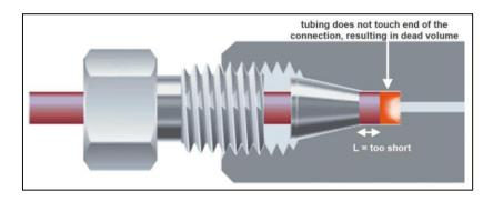
Every ferrule type needs an appropriate length of tubing for connecting it to the type of connection port, depending on the depth of the connection port. Refer to the information provided by the manufacturer for specific information.
