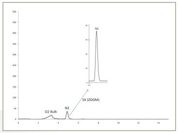
Figure 6: 420 ppb N<sub>2</sub> in O<sub>2</sub> with PlasmaDetek N<sub>2</sub> selective system
