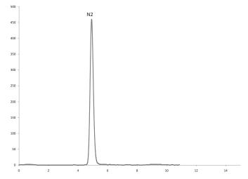
Figure 3: 5 ppm N<sub>2</sub> in H<sub>2</sub> with non-selective detector system
