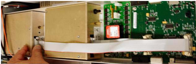
Figure 13 Connecting the APCI HV power supply to the valve PCA.
