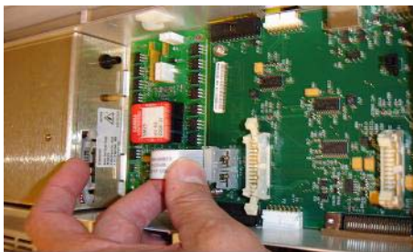
Figure 10 Connecting the valve PCA to the multimode HV power supply.
