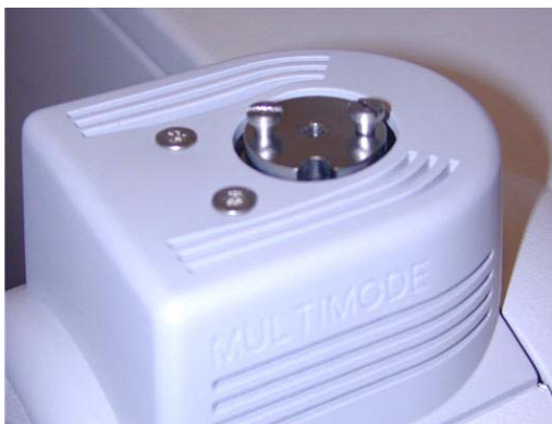
Figure 23 No nebulizer on top of the multimode source
