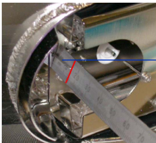
Figure 5 Installing the thermocouple probe and 15 mm adjustment
