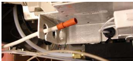
Figure 14 Connecting the APCI HV to the chassis.
