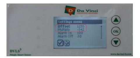
Note:Due to the nature and electronics of the Hydrogen sensor, the Multiply factor normally reads negative (a raw signal drop is observed when Hydrogen is detected).
