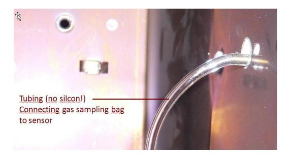
Note:Do <u>not</u> use any <u>silicon</u> hose for connection of the gas sampling bag to the sensor!
