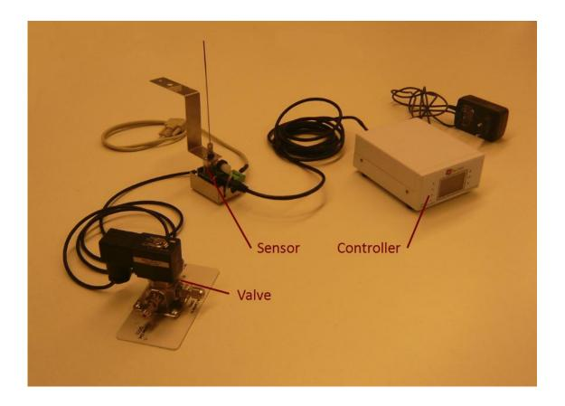
Both the valve and sensor assembly are mounted on the GC, the position depends on the type of GC used. The controller box is normally placed on top of the GC, but may be installed in the near area as well. A hardcopy of the user manual is included as well.
