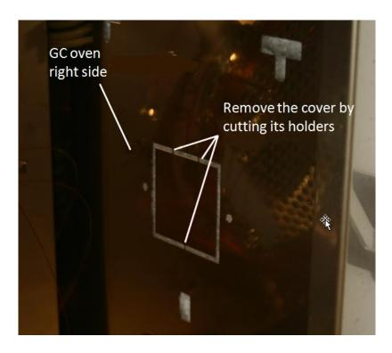
Carefully create a small hole in the oven insulation to allow for the sensor tube to be inserted.
