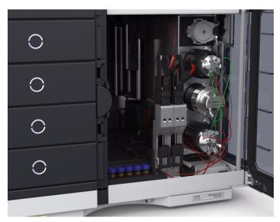
Multisamplers G7167A/B are optionally available with a second needle. This unique Agilent feature offers access to two great new possibilities: In alternating needle mode, a Smart Overlap function allows drawing the next sample while measuring the current sample. This reduces cycle times strongly while minimizing carry-over to lowest levels by flushing the alternative flow path in parallel.
