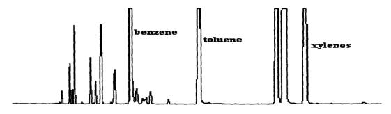
Air sample desorbed using OPTIC, without cryogenics.
