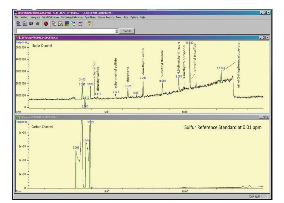
Figure 2a. Sulfur Reference Materials Chromatogram at 0.01ppm
