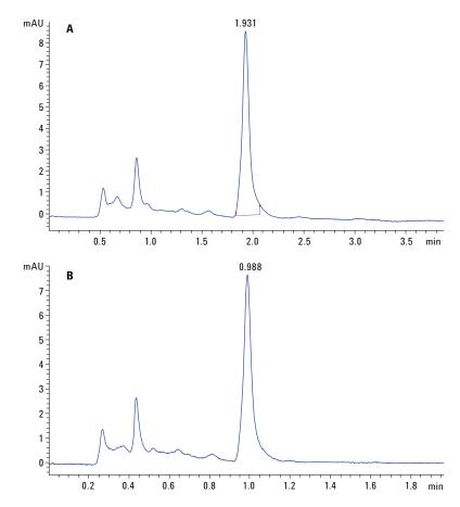
Figure 6. Improved efficiency by means of a shorter column  $(3.0 \times 50 \text{ mm}, 2.7 \text{ µm} \text{ at } 0.43 \text{ mL/min})$  and higher flow rates. A) Reduction of column length to one third reduces the elution time of caffeine to 1.93 minutes, run time to 4 minutes, and increases sample throughput three times. B) Doubling the flow rate to 0.86 mL/min reduces the run time to 2 minutes and the elution time of caffeine to 0.988 minutes.
