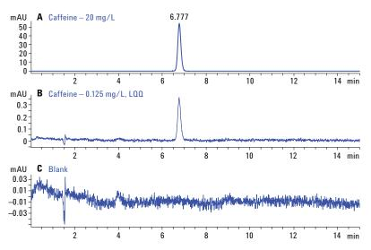
Figure 3. Determination of carryover of caffeine for the maximum concentration used. A) Maximum concentration of caffeine at 20 mg/L. B) Lowest level of caffeine used for calibration at 0.125 mg/L (LOQ = 0.051 mg/L), as comparison. C) Blank injection following maximum caffeine concentration injection showing no carry over.
