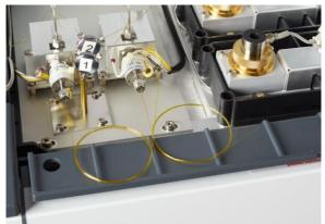
Figure 1: Heated valve unit.
