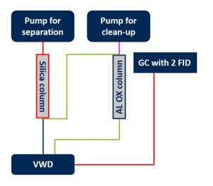
**Figure 4:** Schematic structure of online aluminum oxide purification.
