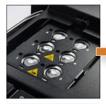
The sample vial is incubated/agitated to speed up analyte equilibration.
