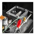
If applicable, the trap is thermally desorbed at up to 100°C/s to inject the sample into the GC-MS as a narrow band.
