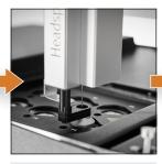
Headspace vapour is withdrawn. Overlap mode optimises productivity for the incubation & sampling of multiple HS vials.
