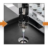
The probe is removed from the vial, and a wash/dry station removes residual sample matrix.
