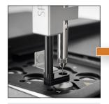
The SPME fiber is normally positioned in the sample headspace and incubated/agitated to facilitate extraction.
