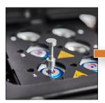
The robot inserts the probe into the vial, and the assembly is incubated/agitated to ensure analyte equilibration.
