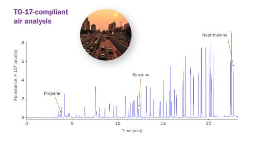
**This analysis of a 5 ppb 65-component VOC standard** demonstrates the ability of Centri to monitor a wide range of 'air toxics' in accordance with US EPA Method TO-17.
