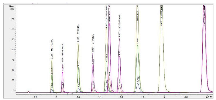
Overlay of multi-component calibrator mix - 0.01%, 0.05%, and 0.10% Conc.
