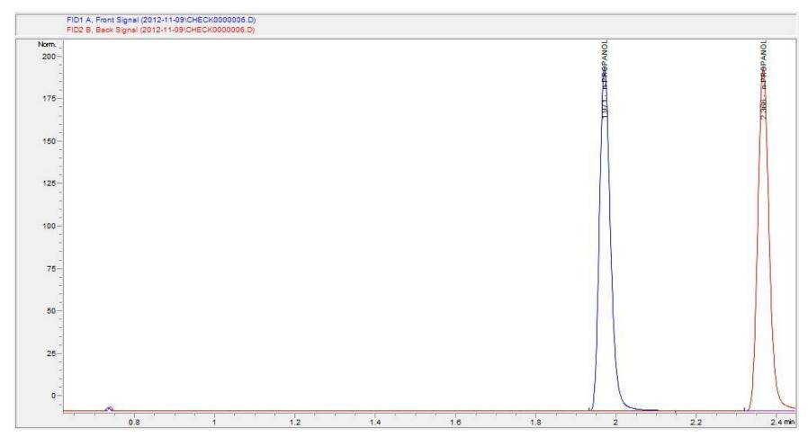
System blank run after 0.50 % ethanol control, n propanol ISTD
