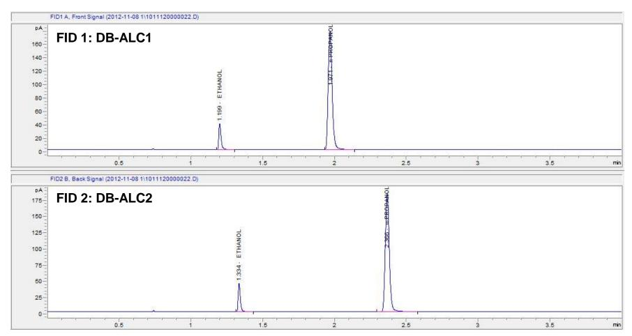
Ethanol control sample (0.05% conc.) with n-propanol ISTD
