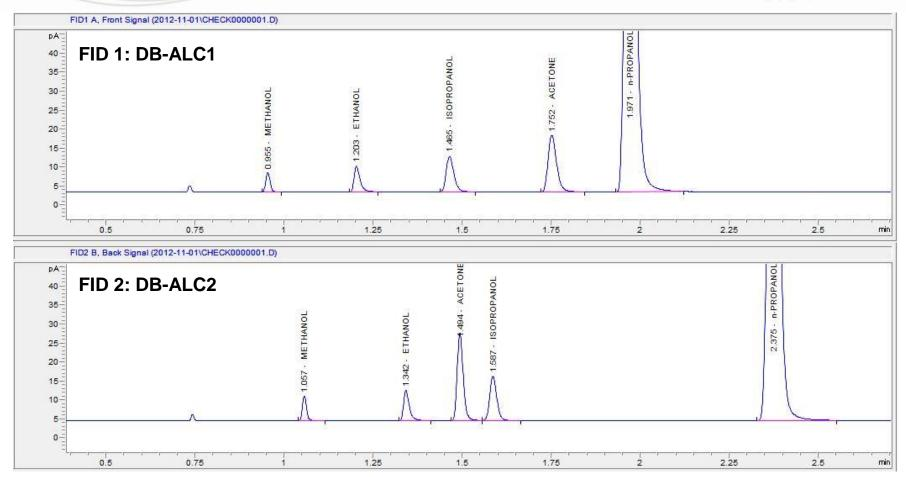
Ethanol and mixed volatile calibrator, n-propanol ISTD
