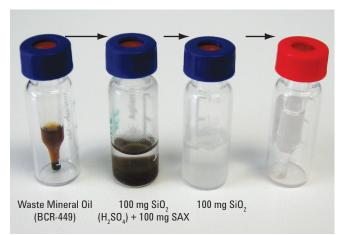
Fiaure 2. Picture of 2-mL vials during different clean-up steps on an Agilent 7696 Sampe Prep WorkBench.
