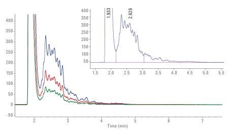
Figure 5. Chromatogram of the diesel sample (blue) and its 1:1 (red) and 1:3 (green) dilution; the inset on the right shows the setting of the integration marks corresponding to the PFM.
