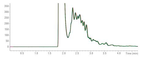
Figure 6. Overlay of 10 chromatograms of a diesel sample.
