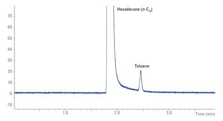
Figure 2. Chromatogram detail of a solution with 0.1 mass % toluene in hexadecane  $(n-C_{15})$ .
