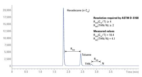
Figure 3. Determination of the resolution values for RNM (hexadecane to toluene) and RMD (THN to N) using the performance mixture.
