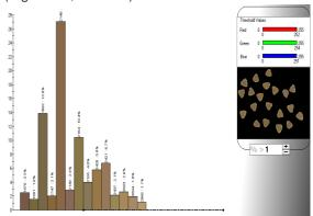
Figure 11: Color spectrum of the Lycat pet food obtained with IRIS system
