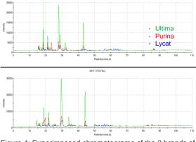
Figure 4: Superimposed chromatograms of the 3 brands of Pet food, obtained with HERACLES NEO e-nose
