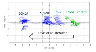
Fig.4: Odor map of orange juice samples based on principal component analysis (PCA) using selected volatile compounds of Heracles e-nose
