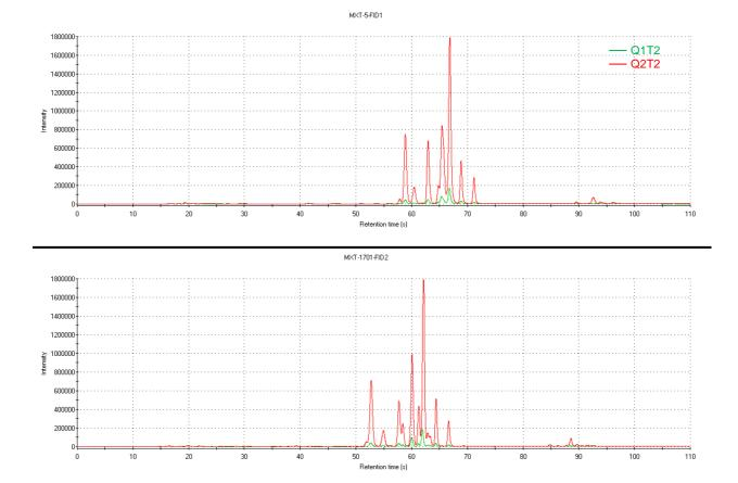
Fig.2: Chromatograms of a contamination-free pepper (Q1T2) and a pepper contaminated with mineral oil (Q2T2) obtained with HERACLES e-nose
