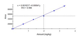
Fig. 2: Calibration curve of 1-vinyl cyclohexene in plastic (MXT-5 column)
