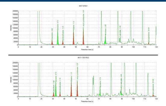
Fig.5: Composition analysis (in mg/kg) of volatile contaminants of HDPE with limit interpretation (green for pass and red for fail)
